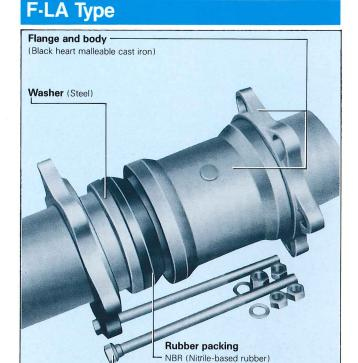
As shown in the photo, the F-LA type consists of the body, rubber packings, washers, flanges, bolts and nuts. Highly elastic rubber packings are pressed against pipe ends to seal the fluid. The high elasticity of rubber packings exerts a large reaction and frictional force on the flange so that bolts and nuts do not loosen. Pipes should be fixed.
