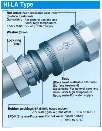
HI-LA type is one variation of the LA type with lock rings provided to prevent pipes from slipping off.
