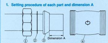
Each part should be set in numerical order as shown in the figure. At that time, rubber packing should be set conforming to dimension A as listed in the following table.
