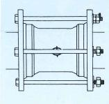
In case of F-LA type, tighten the bolts and nuts by hand, then tighten symmetrically with a spanner according to the value of tightening torque as listed in the table.
